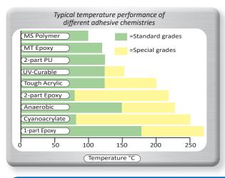
Hot strength of Permabond anaerobic adhesives:
