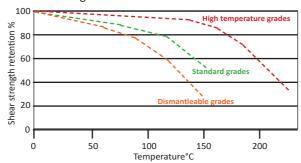
The temperature range the joint will be exposed to is an important factor in deciding which adhesive to use. Adhesive strength reduces as temperature increases, as demonstrated in the graphs to the left and above. Provided adhesives are kept within their recommended temperature range, full strength should be regained upon returning to room temperature.
